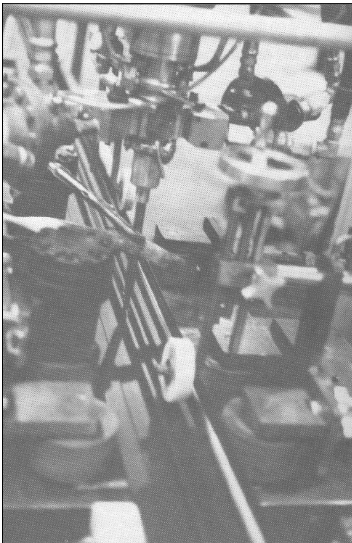
FIGURE 15: Pouring of Thermal Barrier
