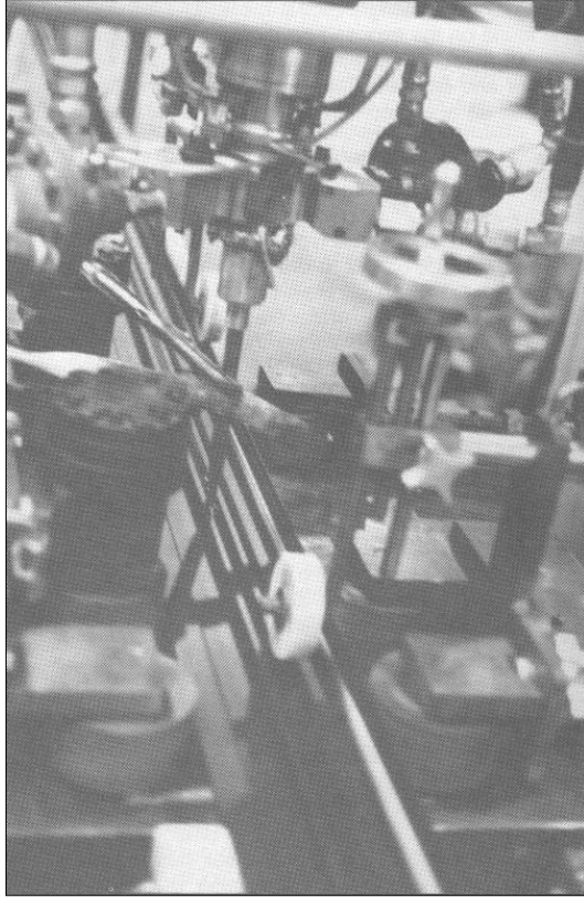
FIGURE 15: Pouring of Thermal Barrier
